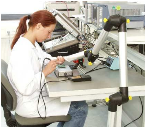
Figure 5: Extraction arm for pollutant capturing at work place
