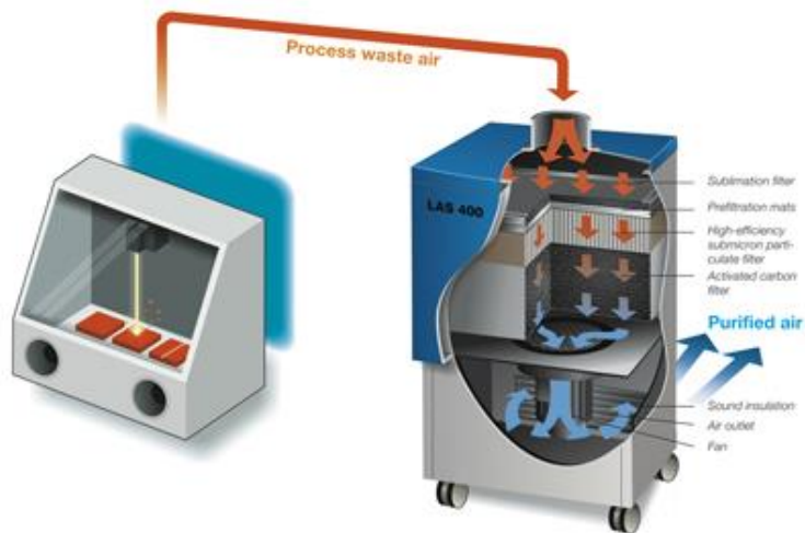
Figure 3: Example for combinational filter in an extraction and filtration system for laser processes
