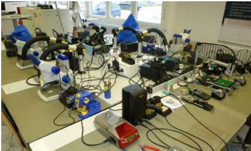
*Image 3: Manual workplaces with installed extraction arms*
