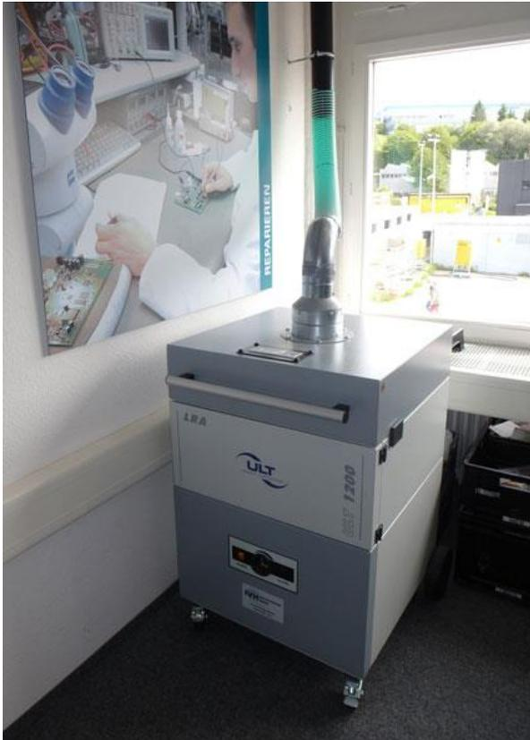
*Image 4: LRA 1200 utilized as central extraction system for soldering fume*
