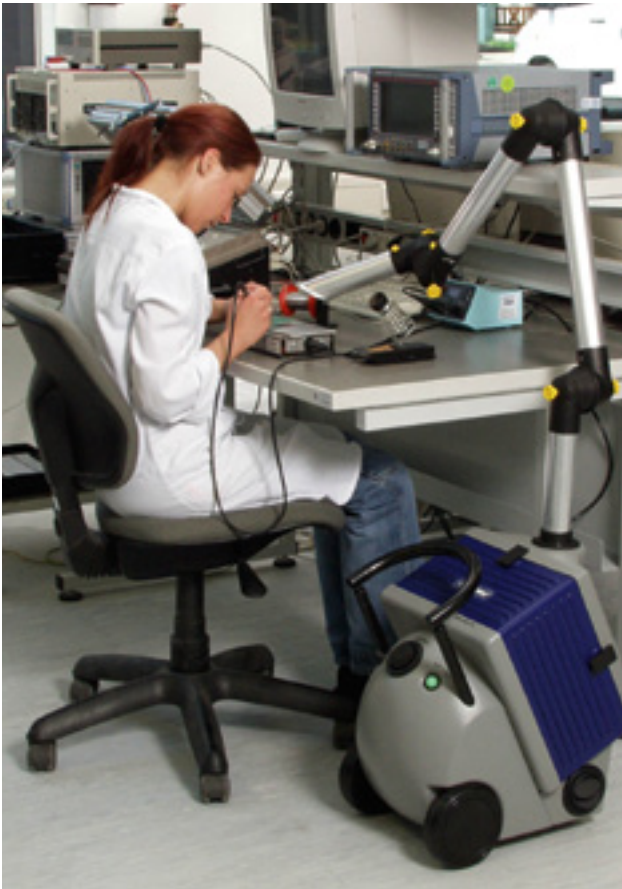
Manual soldering workstation with fume extraction technology.
