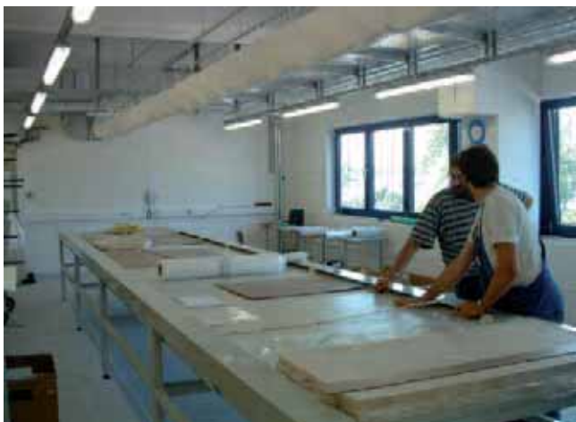
Fig. 1. Cutting of glass mats to size
